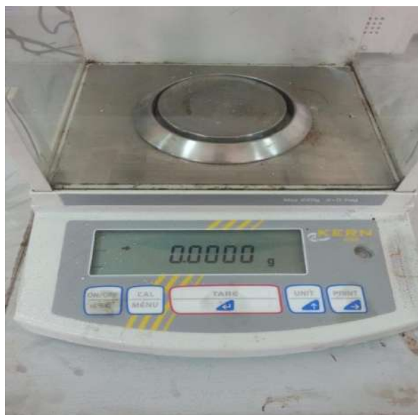
Figure (4.15) Sensitive Balance with an Accuracy of (0.0001g)
