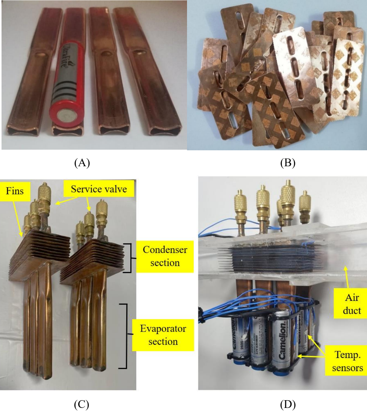
Figure (4.10) Photograph of the HP-Model: (A) copper tube of the HP, (B) fins, (C) HP after fabrication, and (D) HP with Li-ion battery connections.
