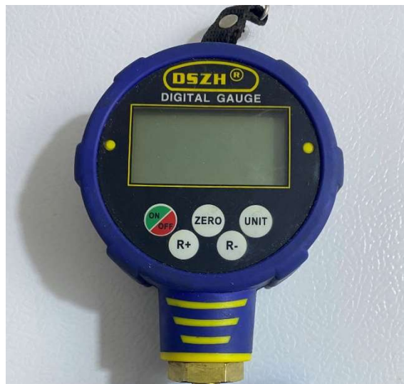
Figure (4.11) Digital vacuum pressure gauges.
